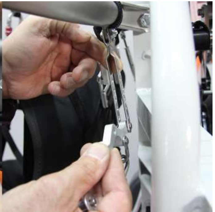
Attach the left cable and using the tensioning device pull the cable tight.
