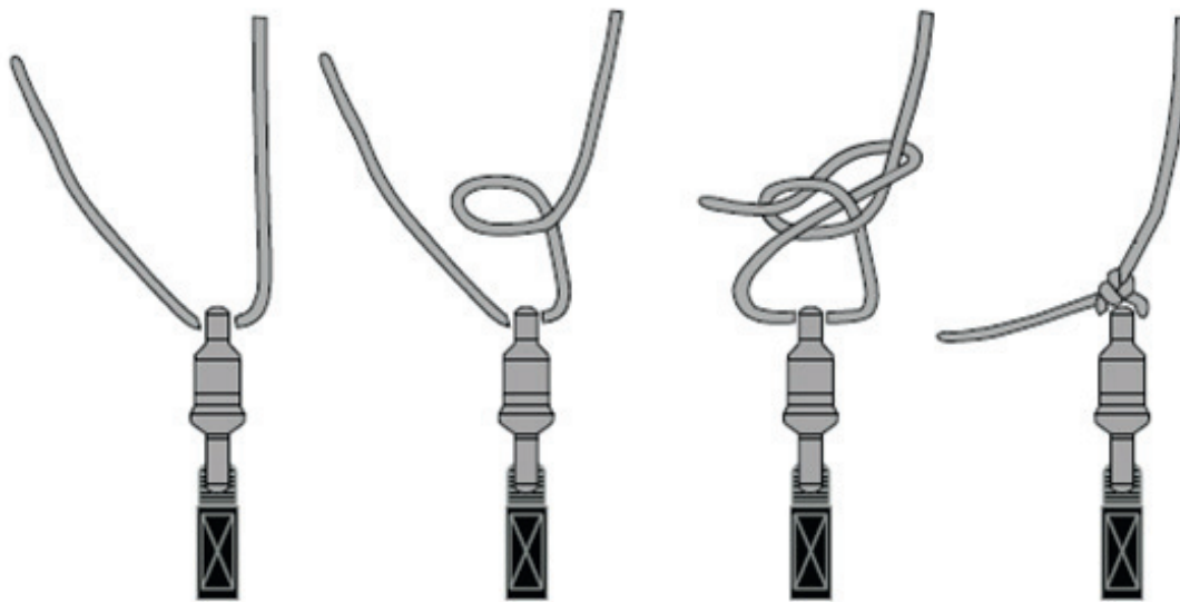
Figure: Bowline knot
