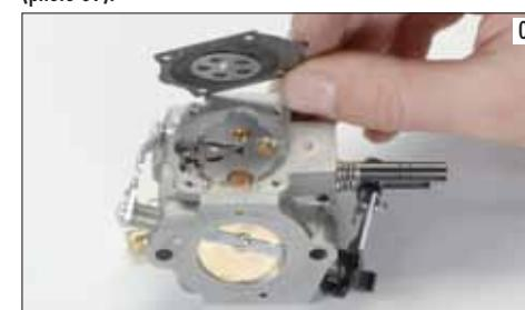
**ATTENTION:** The carburetor is made of many small and fragile parts. Be very careful during all the phases with particular attention to the idling and its springs; they both must not be touched.
