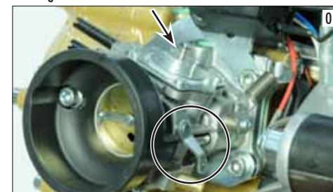
**WALBRO WG8 CARBURETOR (Thor 130 engine only):** Move the starter level to the off position (photo 1); now hand the starter and start pulling the rope till it grows hard. Pull with strength without accelerating till the engine seems to start working (do not repeat this operation more than 3 times otherwise the engine may flood). Now move the starter lever to the on
