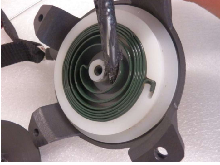
Grease the lower part of the pulley driver and the internal part of the big spring
