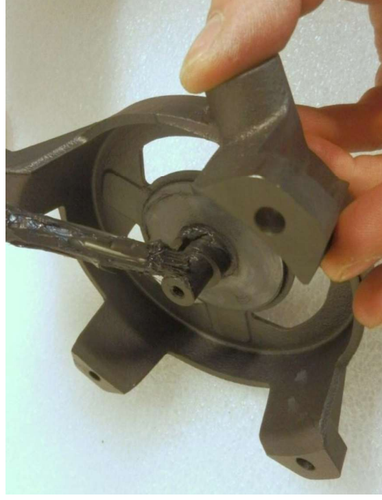
Grease also the upper part of the plastic disk and the central hub of the flash starter, paying attention not to dirty the thread of the hub
