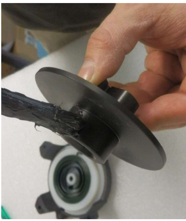
Grease the lower part of the pulley driver and the internal part of the big spring
