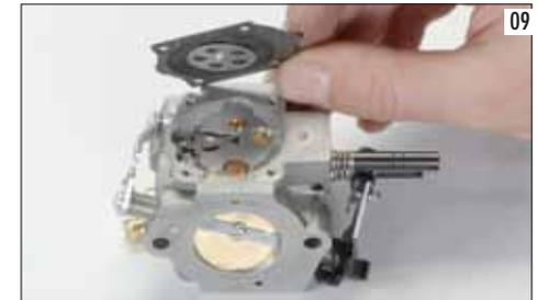
**⚠ATTENTION:** The carburettor is made of many small and fragile parts. Be very careful during all the phases with particular attention to the idling and its springs; they both must not be touched.
