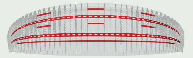
The Vantage 3 achieves both lightness and durability by the intelligent mix of fabric in different locations of the canopy. The same hard-wearing fabric as normal paramotor gliders is used in wear-sensitive locations of the canopy, and lighter but still durable fabric is used in less critical areas such as the under surface.
