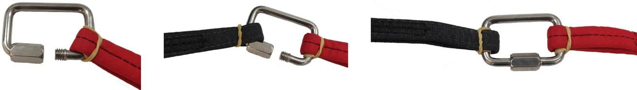
**⚠ WARNING:** *When connecting the rescue bridle be sure to secure the connection using tape, rubber bands or heat shrink wrap. If the lines are not secure they may burn or cut from excess friction.*
