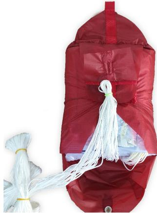
**Fold 60cm of line under the rescue. Secure the suspension line using the central elastic band.**
