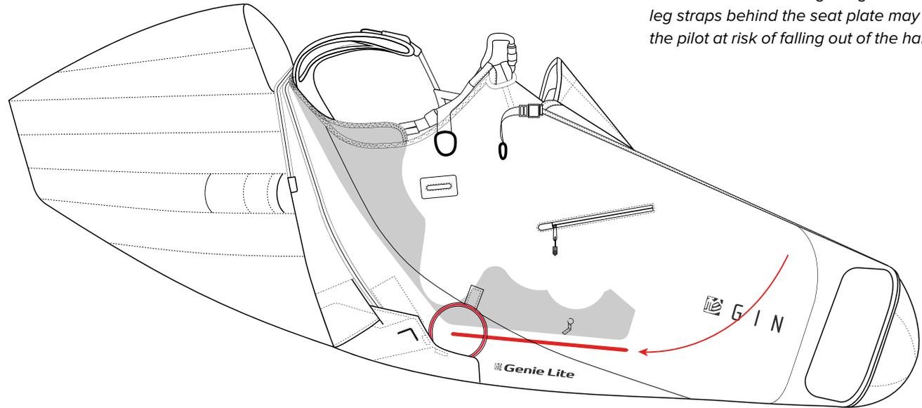
**WARNING:** Forgetting to loop the leg straps behind the seat plate may place the pilot at risk of falling out of the harness.
