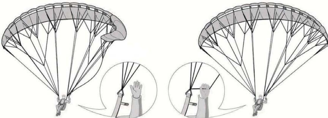
Figure: Grabbing the stabilizer/winglet main line
