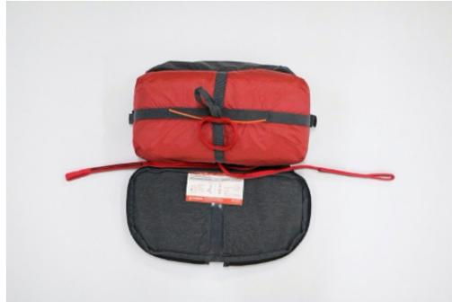
Put the rescue bridles in the bottom of the rescue deck, with one end going out on each side
