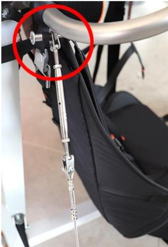
Start with the right rod locking it with the push-pin and then hook the left tie-bar tightening the lever until the holes to be fitted match the push-pin
