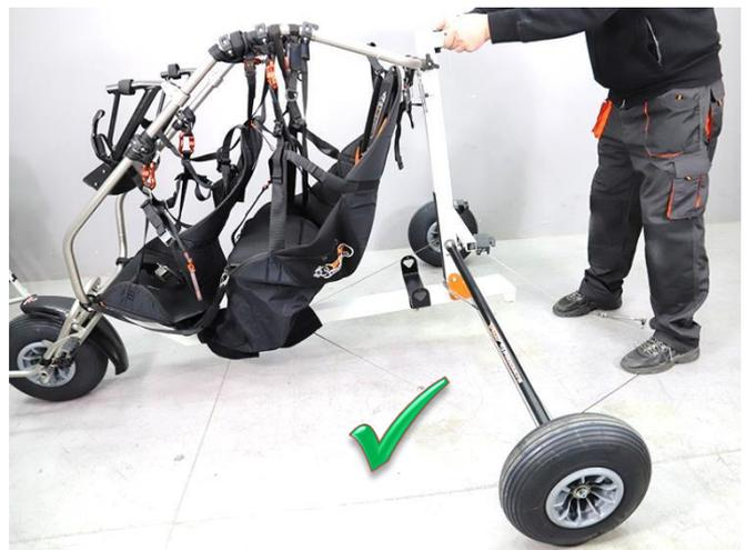
Lock the wheels in place using the lower tie-rod with the elastic:
