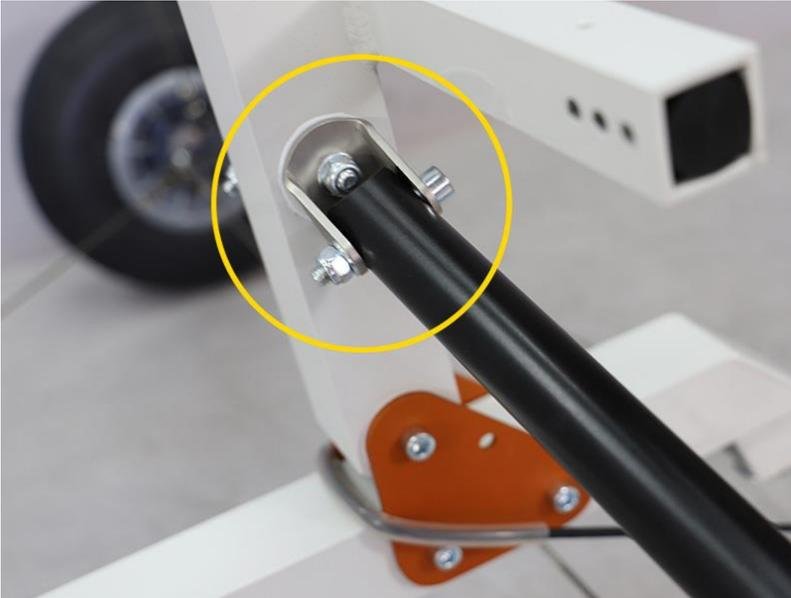
Check the wear and oxidation conditions of the bolts of the rear wheel arms, if they are not in good condition, do not hesitate, replace them immediately!
