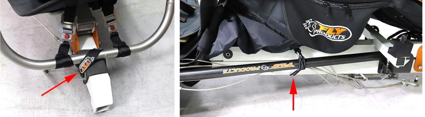
Then lift the cradle and raise the paramotor's coupling support in a vertical position, join the cradle to the support using the special butterfly screw:
