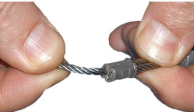
Check the wear and the oxidation conditions of the steel cables of the rear wheels, if they are not in good condition, do not hesitate, replace them immediately!
