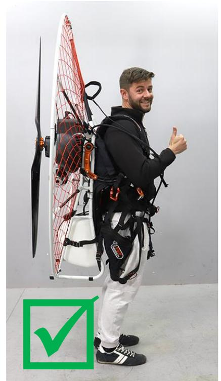
Adjust the paramotor on the shoulders in vertical position
