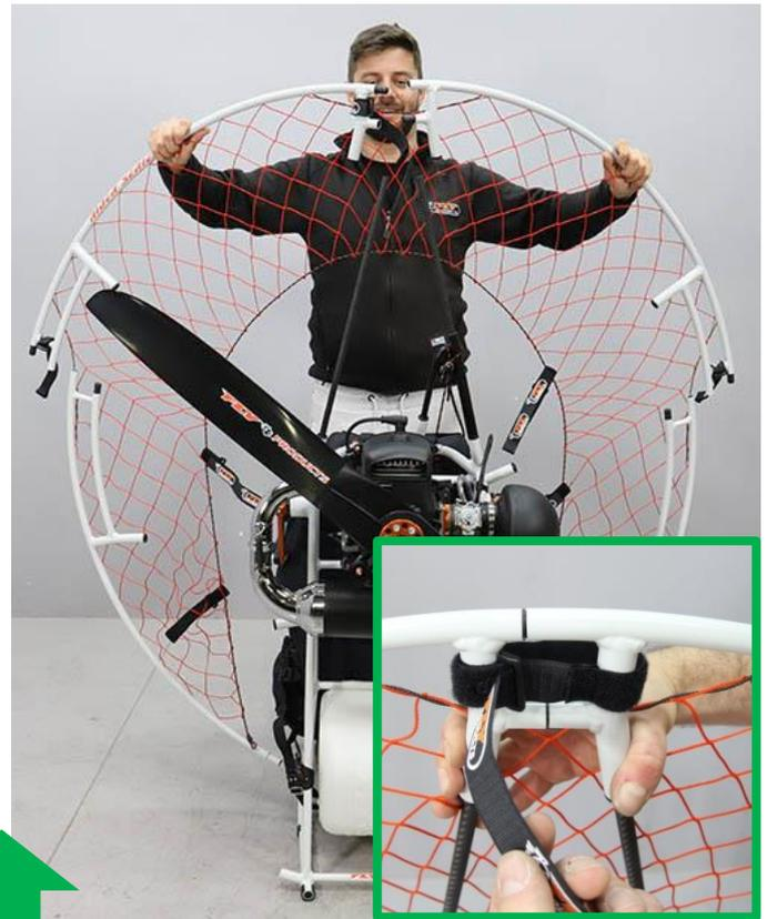
insert the two long rods (A) in the frame and then fit the two upper parts of the cage, hook them together and close the Velcro strap to lock them.
