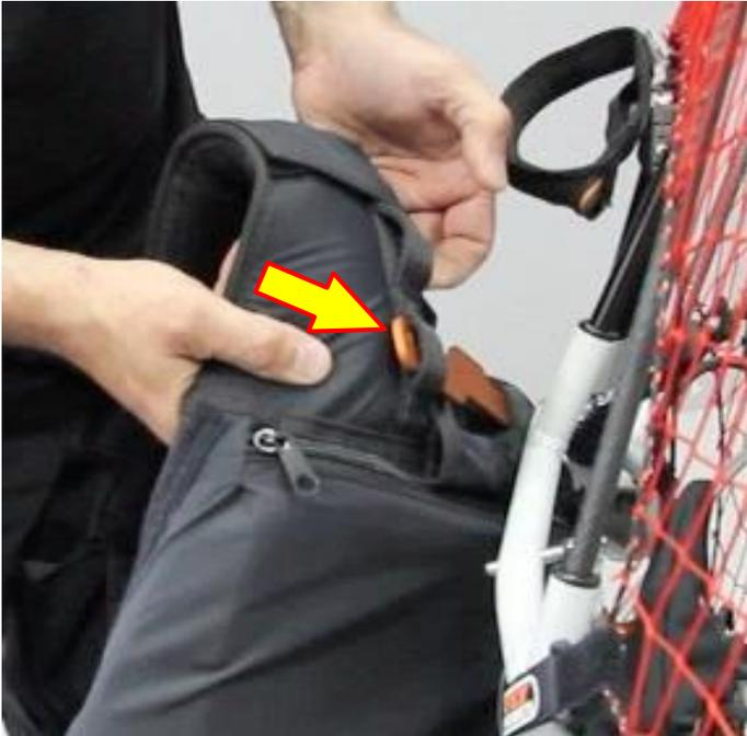
insert the harness on the prepared plate and lock the push-pin
