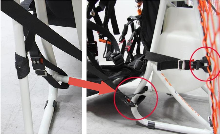
Hook the four lower straps onto the quick-lock provided bucklets
