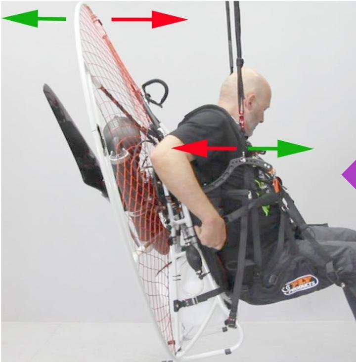
This setting has effect on paramotor inclination in flight: moving the hooks forward the paramotor inclines backwards and vice versa.
