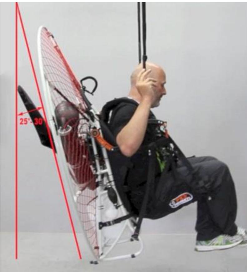
Before you make the first flight try the position. Hooks the paramotor and test the inclination which must be between 25° and 30°. To be comfortably seated the harness has many adjustments through which you can find your best position.
