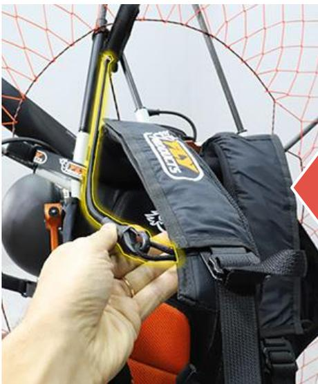
Hook the elastic rope of the starter handle to the prepared eyelet and lock it under the velcro for 5-10 cm.
