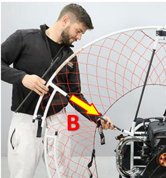
Insert the MEDIUM rod (B) first on the external cage and then on the frame pushing well for a correct engagement
