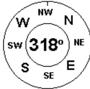
The Compass element show all the data provided by the VARIO M built in magnetic compass. The compass includes an red top arrow which is always aligned with the VARIO M . If the VARIO M is turned the cardinal points will also turn in order the arrow tip points the right cardinal point.
