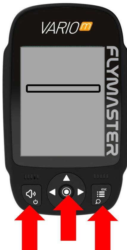
If for some reason your instrument does not start and keeps rebooting without any apparent reason, it's possible to put it in “recovery mode” so the firmware can be restored via Flymaster Instrument Manager.
