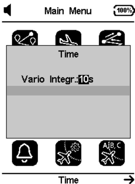
**Vario integrator** - The Integrated vario is calculated by integrating the vertical speed during a period of X seconds defined by this value. In the example, the integration period is 5 seconds (default value).
