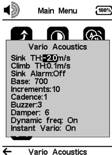
The Vario Acoustics settings menu option allows the user to change vario sound related parameters. The user can change the climbing, and sinking rate sound through the respective threshold values. These thresholds correspond to the climbing and sinking rates at which the sound activates. The user can also define in the the Acoustic Thresholds option the sink alarm and the sound volume of is the VARIO M.
