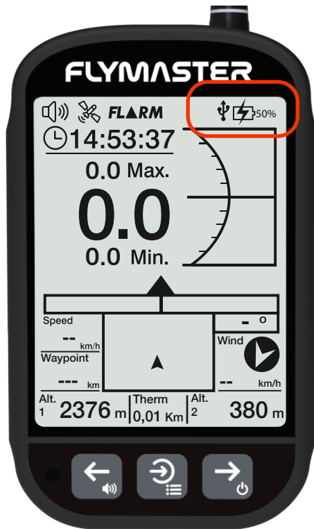
The LS2 GPS is charging from an external power source while powered on.
