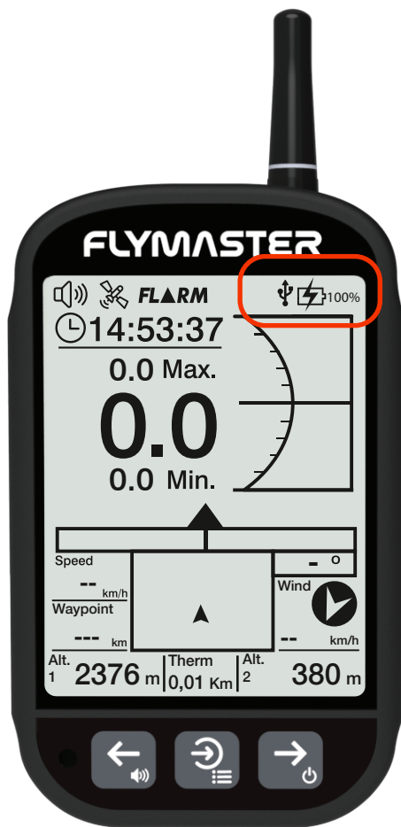
The LS2 GPS is charged from an external power source while powered on.
