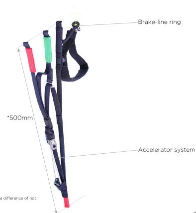
\*For certification, the riser length of the test sample may have a difference of not more than 5mm from that specified here
