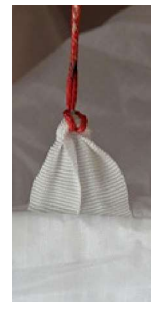
Looped junction – incorrect
