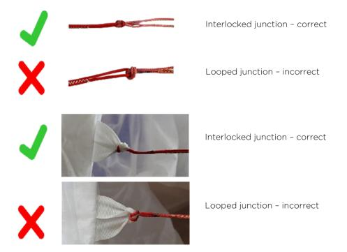
After rigging the wing, always do a full dimensional check of the lines, and inflate it to ensure that everything is correct before flying.
