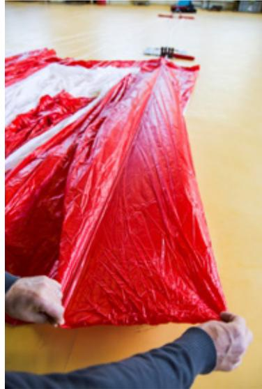
*Pic. 50* Lay panel #4 to the outside and halve it (one fold)
