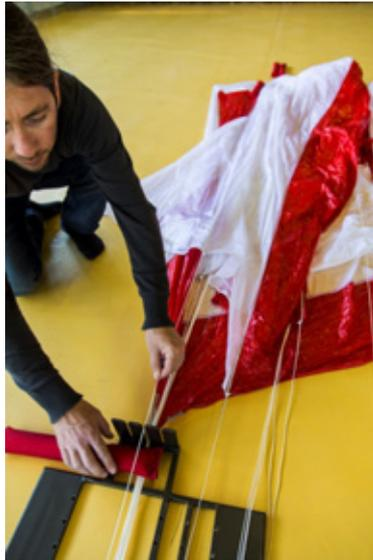
*Pic. 41* Put the panel #2 line in the line separator
