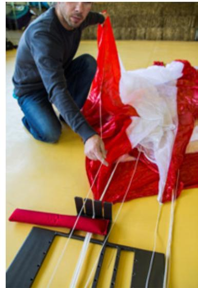
Pic. 33 Put this line in the line separator (weight)
