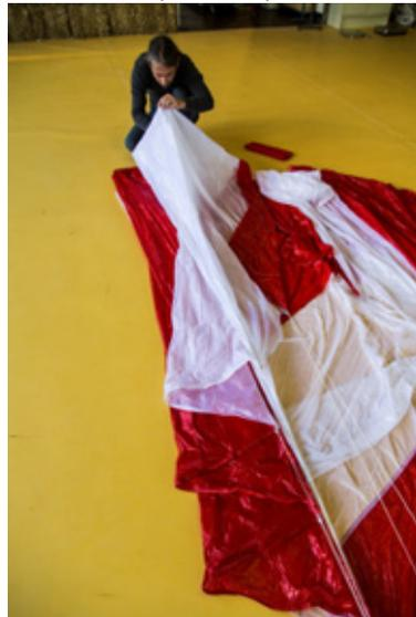
*Pic. 53-55* Fold the remaining panels up to the nose...
