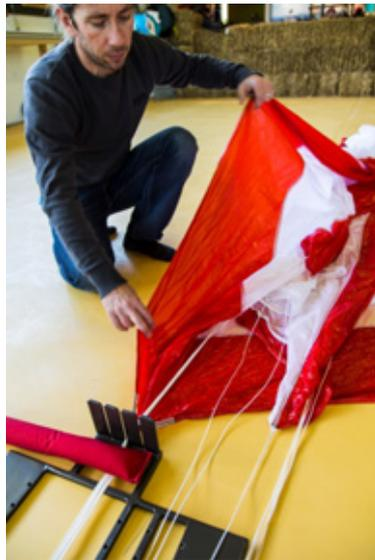
Pic. 32 Go along the bottom edge from the middle line to the first line
