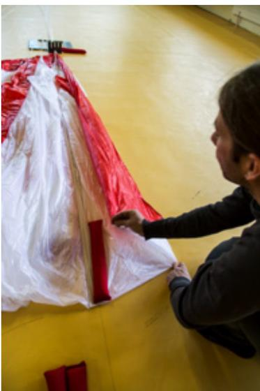
Pic. 37/38 ...with an S - 2 folds (for Beamer 3 small only halved)
