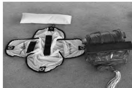
8. We will proceed to introduce the parachute in its container and the subsequent ordering of the lines with the help of rubber bands, finally closing the inner container, being ready for installation in the chair.
