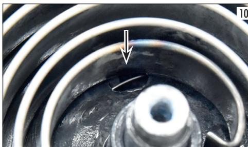
place the springs, the teeth for the starter jaw and screw the cover again using medium thread-locker.
