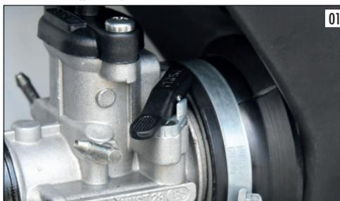
Operate the starter without accelerating till the engine starts. Once it runs switch it off, disconnect the starter and start the engine again slightly accelerating.
