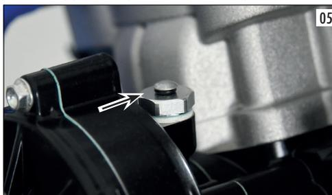
and fill it out with 100cc of ELF Moto Gear Oil 10 W 40 ANTI Clutch Slippage oil. Fit the pipe and its tube again. As an alternative you can use also oil: Shell advance gear SAE 10 W 40 API GL-3 or an oil with 10W40 viscosity compatible with clutch (similar to motorcycle engine oil)
