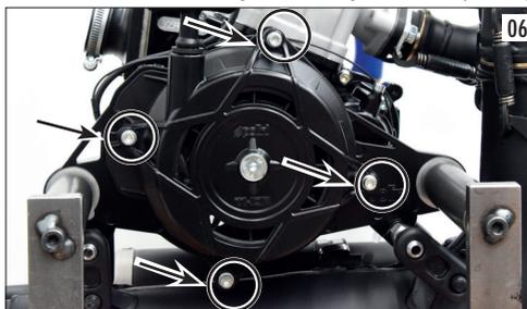
Remove the handle knot. Be careful since the central wheel will spin till the spring is completely discharged: keep it and discharge it slowly to avoid damages or possible injuries. Remove the central screw and its cover (photo 7).
