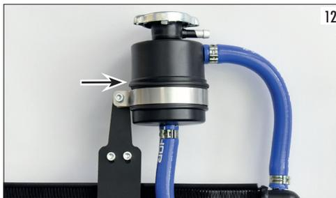
If necessary add some liquid, using the one specific for aluminium radiator.
