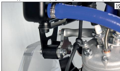
Fit the two rubbers on the bracket and place the radiator. To fix the radiator in the top side a bracket and a rubber are provided.
