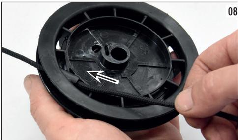
wind up the rope on the wheel (according to the entrance sense of the rope on the wheel) (Photo 9).
