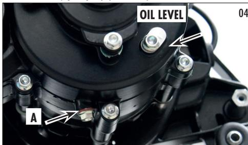
Collect the oil flowing out in a suitable container. Wait till the oil has completely flown out and, if necessary, tilt the engine to the side to make this operation easier. Tighten the screw with strength. Unscrew the breather pipe in the top side of the crankcase (photo 5)
