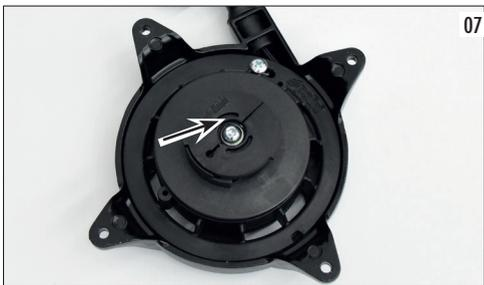
**⚠ ATTENTION!** Under the cover there are two teeth for the starter jaw (check their condition and if worn replace them); under them 2 small calipers. Be very careful not to lose these small parts.
