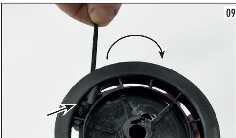
Now insert the plastic wheel in its housing again, and check through the hole that the internal spring hook is perfectly coupled (Photo 10)
