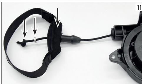
**⚠ ATTENTION!** verify that the return spring does not reach the end of the stroke. Extract the rope completely and turn the wheel again to check that it can make at least one turn before stopping.
