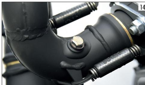
The EGT temperature detected in standard conditions of use should be around  $550^\circ$ - $650^\circ$ , maximum temperature  $680^\circ$ .
