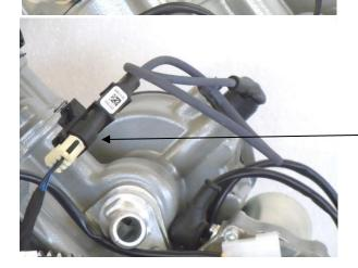
Connect the crank trigger sensor.
