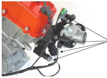
Connect the injector nozzle, throttle position sensor, MAP sensor and the ignition coil to the wiring loom.
