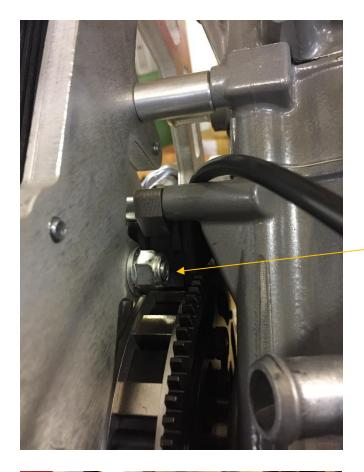
Place the M8 self-locking nut at the back of engine back plate. Don't tighten it yet.
