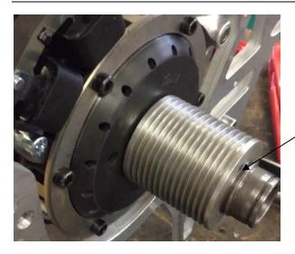
Remove the circlip and the distance shim from the PTO shaft.
