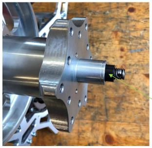
Push the propeller hub back on the propeller shaft.
