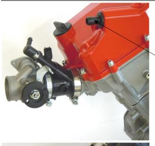
Push the throttle body on the intake port and tighten the clamp. (Use the clamp from the carb rubber)
