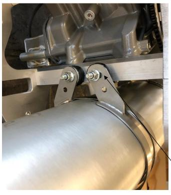
Install the exhaust muffler.
