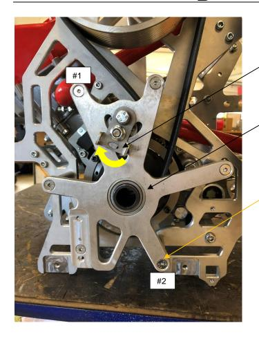
Release the belt tension by moving the belt tensioner lever.
