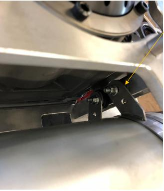
Connect the 2 cradles with the silent blocks below the engine mounts and push the manifold into the exhaust muffler.
