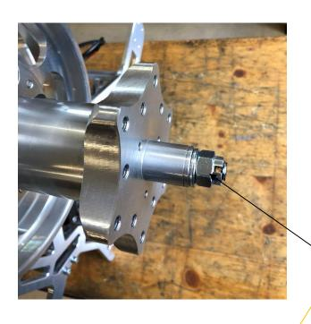
Remove the pin, unbolt the M12 crown-nut.
