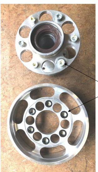
Push the propeller pulley away from the hub.
