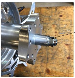
Tighten the M12 with following torque: **40Nm / 30 ft-lb**
