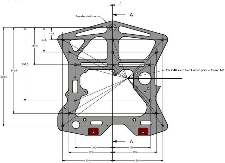
Part shall be fixed to Trike/Quad/ULM chassis with minimum 8 silentblocs ∅ 40 in 68° shore!
