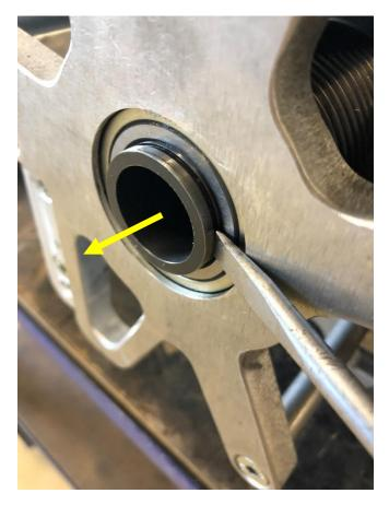
For correct alignment of the clutch drum use a screw driver and pull out the PTO shaft as shown. It should easily move  $\pm$  0,5mm / 0,02 inches.
