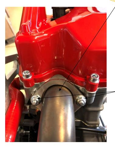
Install the 2 feet and the exhaust manifold.
