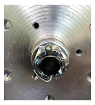
Install the pin as shown.
