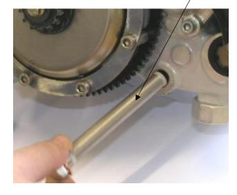
Remove both oil plugs, engine front & oil tank, and drain oil. Clean the magnets of the oil plugs end. Note: In case you observe excessive wear contact your dealer.
