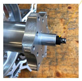
Now it is possible to remove the complete propeller hub from the shaft by pulling.
