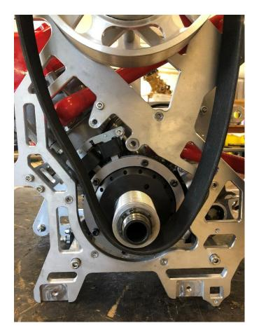
Remove the PTO support plate incl. belt tensioner.
