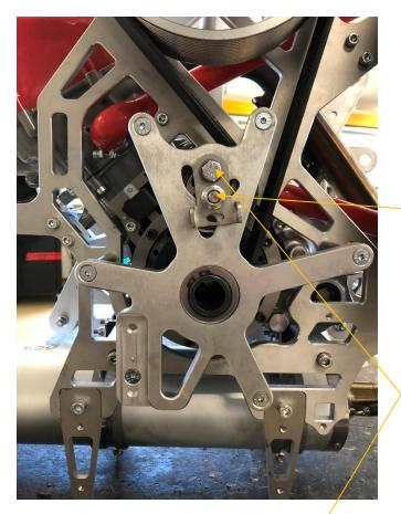
Unbolt the M8 self-locking nut (Don't remove)
