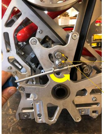
Use a screw driver and place it into the tensioner lever as shown.
