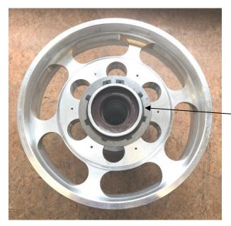
Remove the circlip and the distance shim on the back of the propeller hub.
