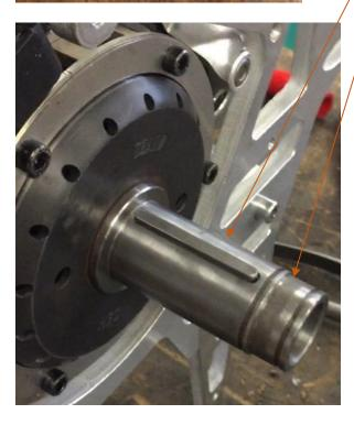
Re-mount distance shim and circlip.
