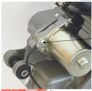
Connect the water temperature sensor.
