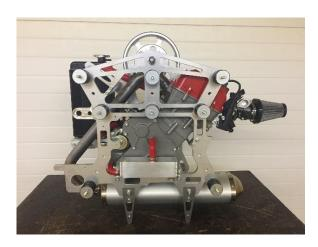
The system comes with 8 pre-installed silent blocks on the front plate. These are the fixation points to install the AERO1000 system on your vehicle! You can change the position of the silent blocks on the front plate. Below you find the dimension sheet!
