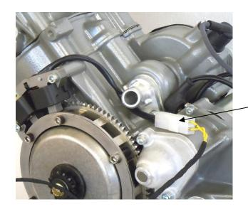
Connect the generator stator to the wiring harness.
