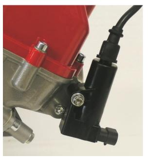
Install the ignition coil as shown.
